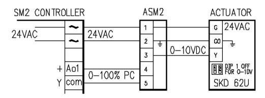
The ASM2/10V converts STAEFA's phase cut signal (0-100%) to a 0-10VDC output signal to drive Siemens valve actuators. The ASM2's phase cut input is optically isolated configured to accept the phase cut (+) & (Y) signal, the output signal is referenced to terminal 2 of the 24VAC/DC input.
