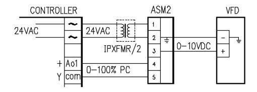
The ASM2/10V converts STAEFA's phase cut signal (0-100%) to a 0-10VDC output signal to drive a VFD. The ASM2's phase cut input is optically isolated configured to accept the phase cut (+) & (Y) signal, the output signal is referenced to terminal 2 of the 24VAC input which should be transformer isolated from the 24VAC powering the controller to avoid ground loop and/or noise problems generated by the VFD.
