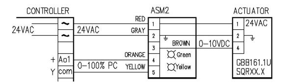
The ASM2/10V converts STAEFA's phase cut signal (0-100%) to a 0-10VDC output signal to drive Landis or Belimo damper actuators. The ASM2's phase cut input is optically isolated configured to accept the phase cut (+) & (Y) signal, the output signal is referenced to terminal 2 of the 24VAC/DC input.
